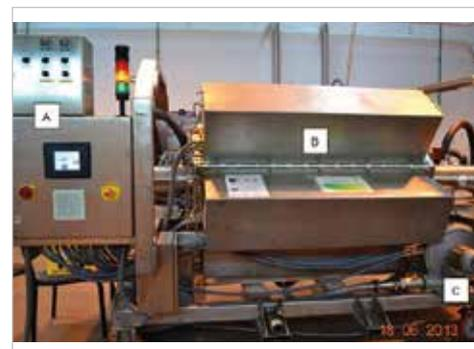
Fig. 2 Side view of the Pentagonal Microwave System. A: control unit for all setup parameters; B: 1 of 5 in pentagonal configuration aligned longitudinal set of 3 magnetrons under a cover; C: fan for blowing heated air and steam through microwave tunnel.
