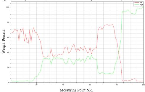
Supposable different intermetallic phases do exist in the welded joint. The distribution over the whole welded joint shows the increase of aluminium and is caused by an accumulation. The overview in Figure 18 and the hardness test by Vickers confirms this theory. The results of the hardness show that the aluminium alloy is softer than the magnesium because it needs heat treatment for hardening (Figure 19).
