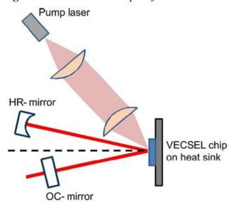
**Figure 4.** Functional Principle of a Disk Laser<sup>[10]</sup>
