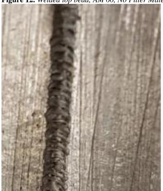
Figure 12. Welded top bead, AM 60, No Filler Material
