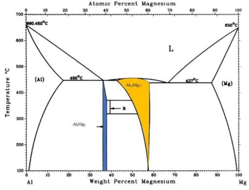
Figure 3. Phase Diagram Al/Mg, Intermetallic Phases
