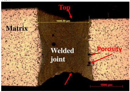
Contrarily to TIG welding, no heat-affected zone appears. To check heat effects in and around the welded joint, Vickers hardness tests were performed. The results of the Vickers test can be seen in Figure 11.
