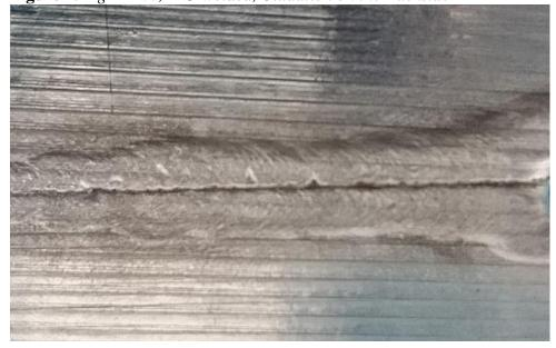
Pulsation plays an important role in all welding processes. In the tungsten inert gas welding process using AC, the pulse current of the welding arc is essential although it is difficult to find the right frequency. If the frequency is too high, the liquidity of the melt becomes too high as well;
