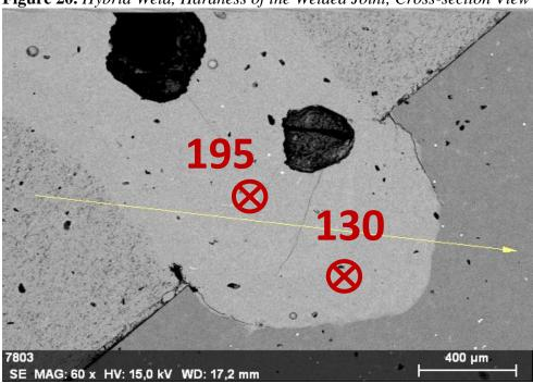
Figure 20. Hybrid Weld, Hardness of the Welded Joint, Cross-section View
