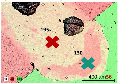
Figure 21. Distribution and Hardness of the Welded Joint
