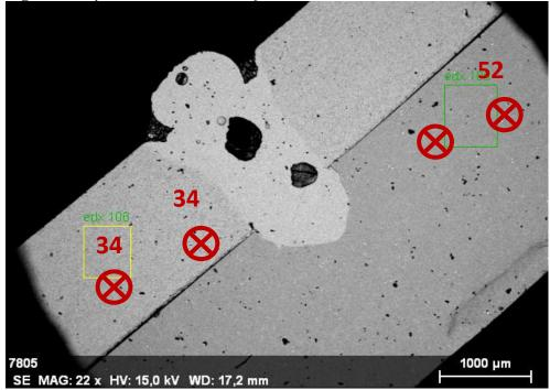
The welded joint itself has a higher hardness than the base materials (Figure 20). In the literature the intermetallic phases between aluminium and magnesium are described as very hard and brittle, so it can be stated that within the welded joint some intermetallic phases had been created, due to previous diffusion processes.
