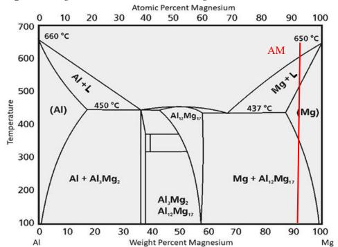
**Figure 7.** *Magnesium-Aluminium Phase Diagram*
