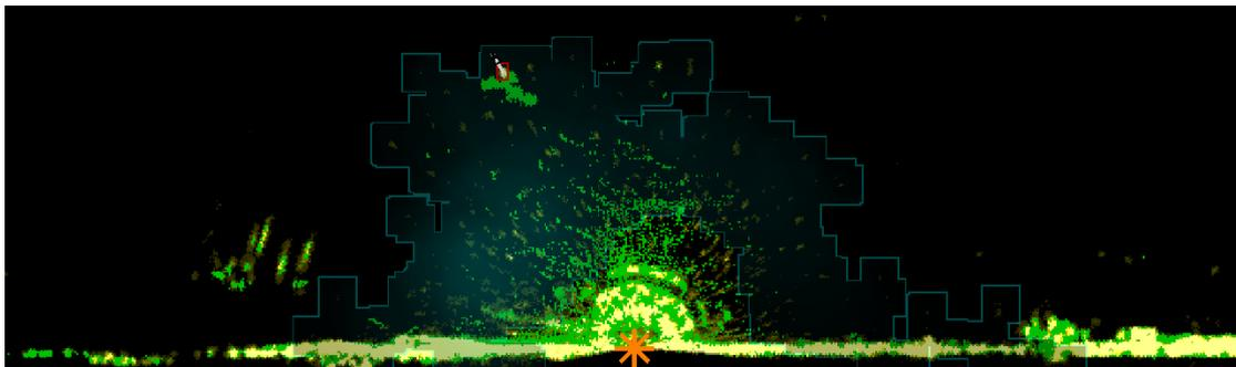
(c) Insect intensity map. The region which seems to be contaminated is highlighted. A strong blue overlay indicates a high contamination level.
