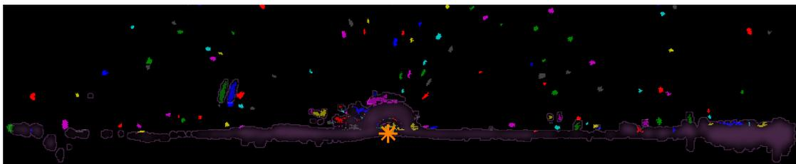
(c) Clutter intensity map and detected echoes. A strong purple overlay indicates high clutter intensity. Detected echoes are randomly colored.
