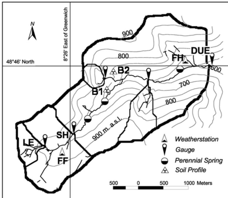
**Fig. 1** Site map and instrumentation of the hydrological test site Duerreych
