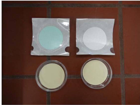
Abb. 5.12: Membranfilter (oberhalb), NKS in Petrischale (unterhalb)
